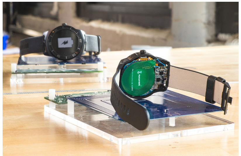
A wearable device charging orthogonal to the transmitter. It illustrates the ability of charging without orientation constraints, which can be important for wearables and other IoT devices that can't guarantee precise alignment during charging.
