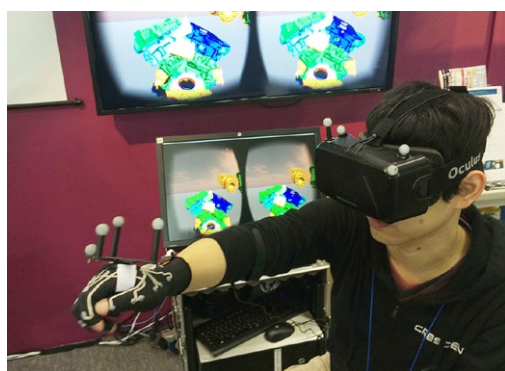
A rugged version of Yamaha’s CNT-based VR gloves with tracking markers for VR applications.
