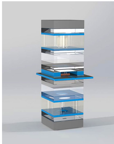
A fully integrated optical microphone concept, showing a dual-side emitting VCSEL in between wafer optics.
