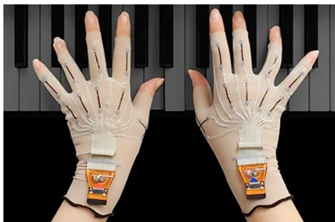
Yamaha’s lightweight and unobtrusive data gloves as demonstrated by a pianist.
